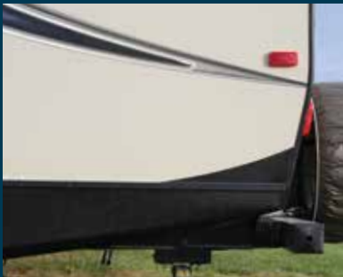
The rear departure angle increases efficiency of windflow underneath and behind the trailer.
