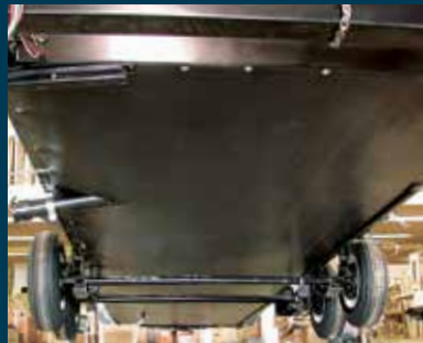
The enclosed underbelly eliminates turbulence caused by exposed frame members, holding tanks, plumbing etc.
