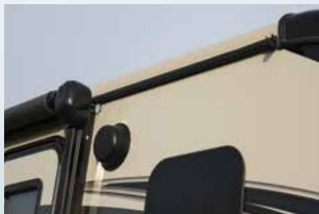
ROLLED ROOF EDGE PROMOTES INCREASED WATER RUNOFF
